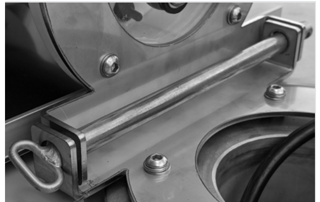
Figure 3: Use the security pin to connect the Ai1 to the top of the DB600. A padlock may be used for extra security.
